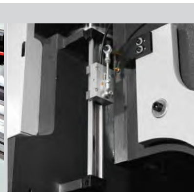
Bending compensation linear scales. Made in Italy
