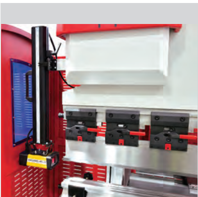
Advanced push button quick release tooling (front load)
